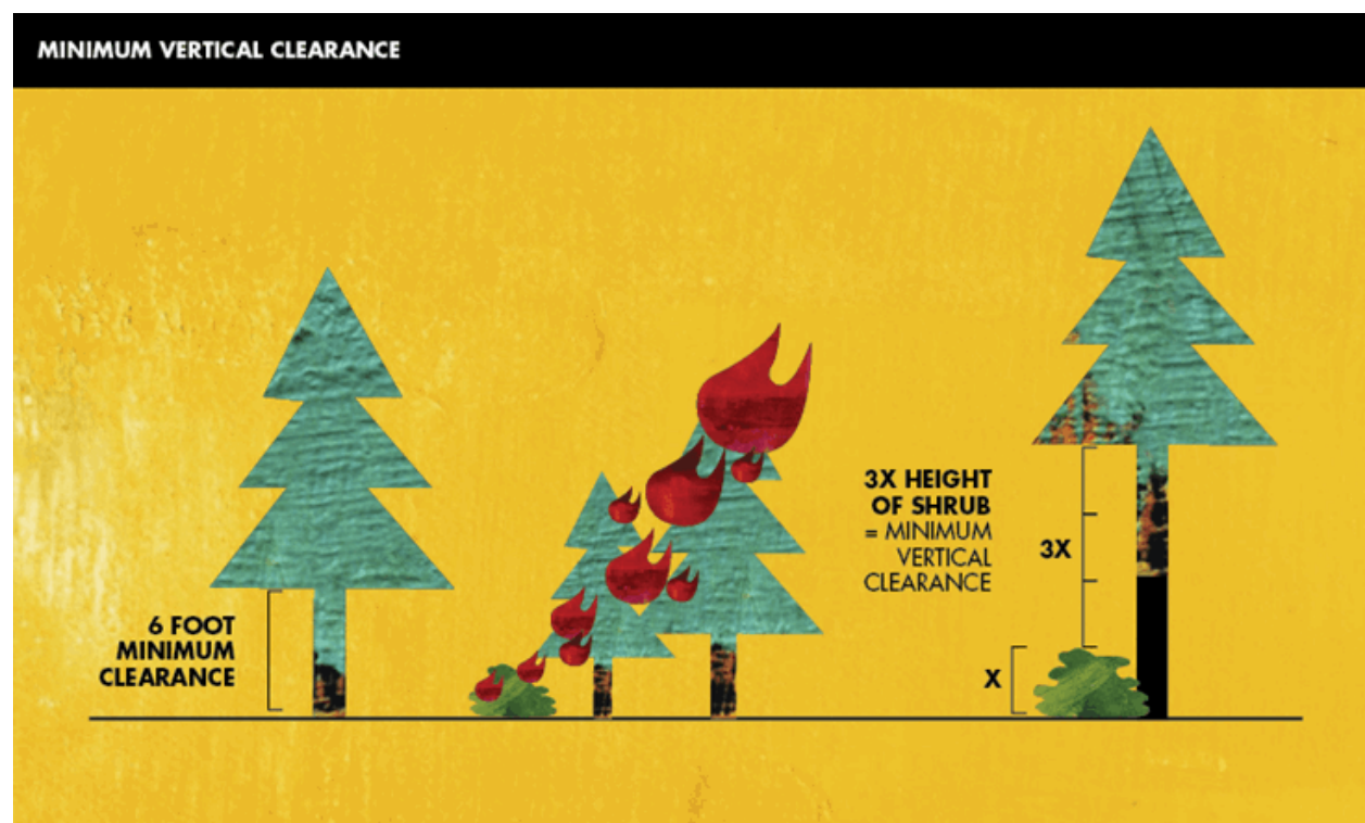
Figure 7: Minimum Vertical Clearance
