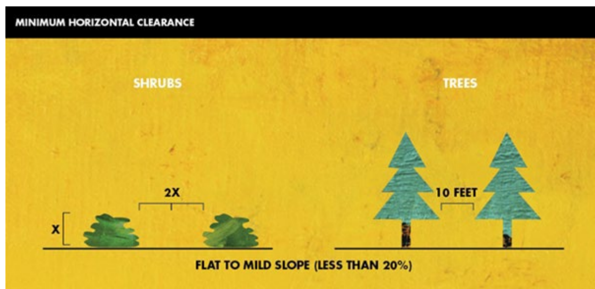
Figure 8: Minimum Horizontal Clearance
