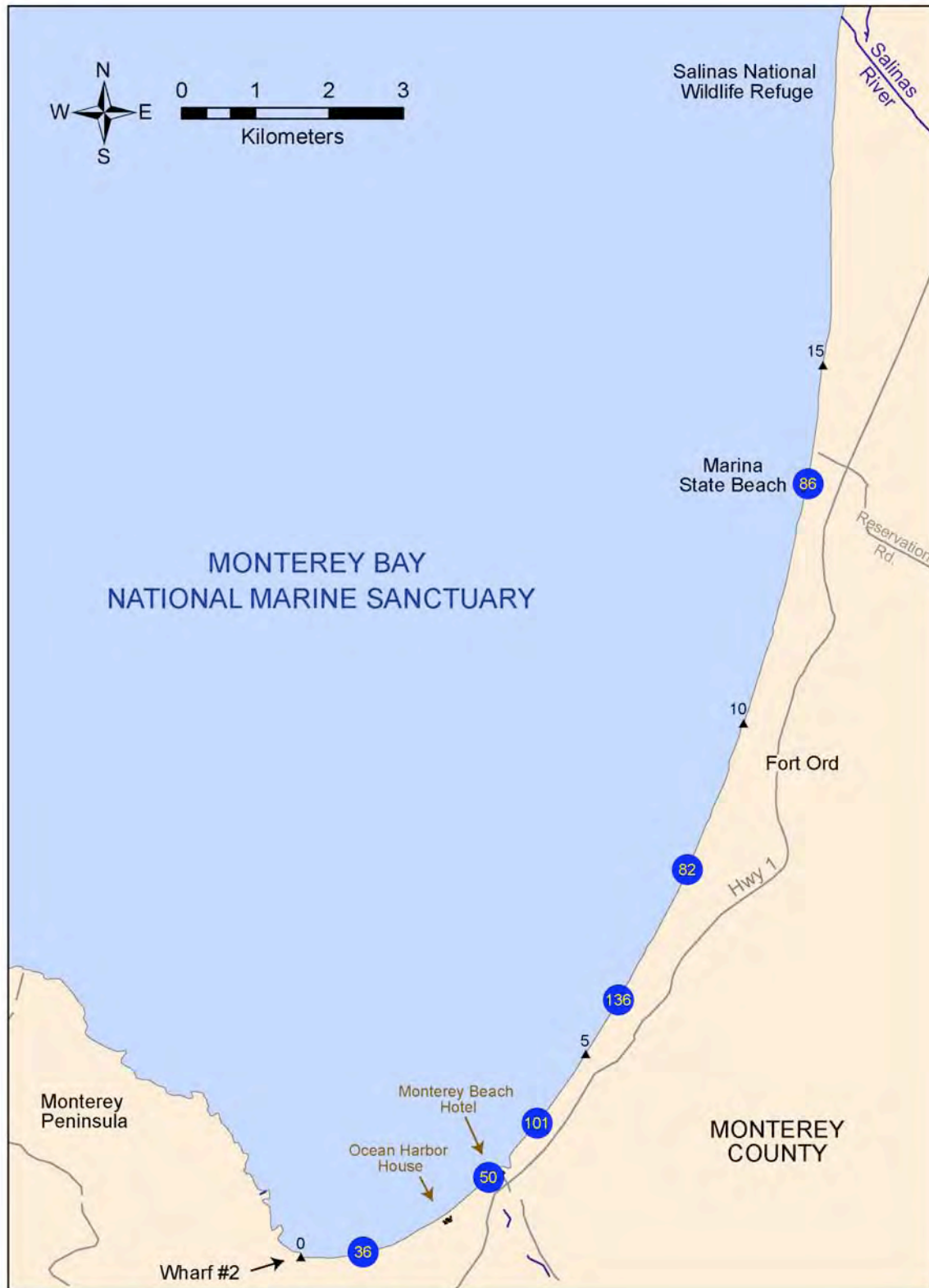
Figure 2.5: Coastal erosion rates in centimeters per year (blue circles) for the time period 1940-2004, averaged from Thornton et al. (in press). Distances from Wharf #2 in Monterey are in kilometers (black triangles). For reference, 100 cm=3.28 ft.
