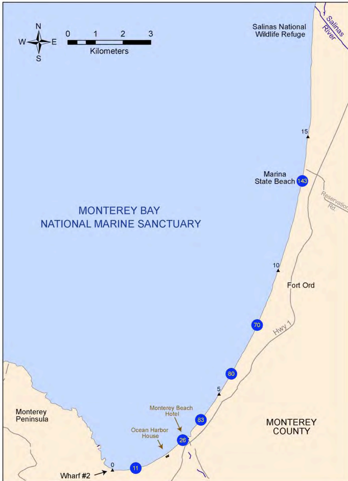
Figure 2.4: Coastal erosion rates in centimeters per year (blue circles) for the time period 1984-2004, as documented by Thornton et al. (in press). Distances from Wharf #2 in Monterey are in kilometers (black triangles). For reference, 100 cm=3.28 ft.
