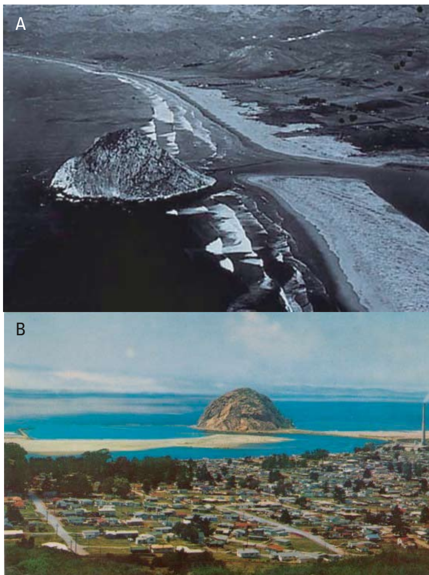
Figure 32. Development of a tombolo at Morro Rock after a causeway was built in the 1930s. Top photo was taken in 1936 just after the completion of the causeway. The postcard (lower image) is from the 1950s and shows a sandy tombolo leading out to Morro Rock (photos: http://morro-bay.com/morro-rock/ ).
