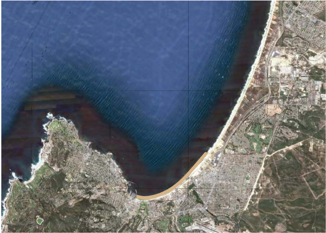
Figure 32 Schematic of Beach Nourishment in Southern Bight
