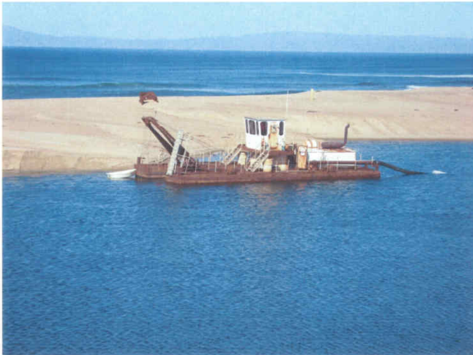
Photograph No. 9. Suction sand dredge situated in the southern end of the material extraction pond adjacent to Monterey Bay at the western edge of the site (viewing northwest).
