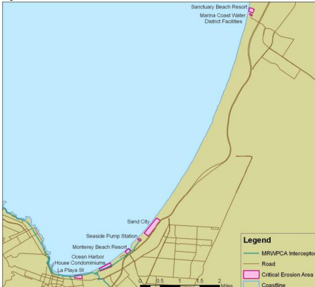
Figure 3: Locations of critical areas of erosion
