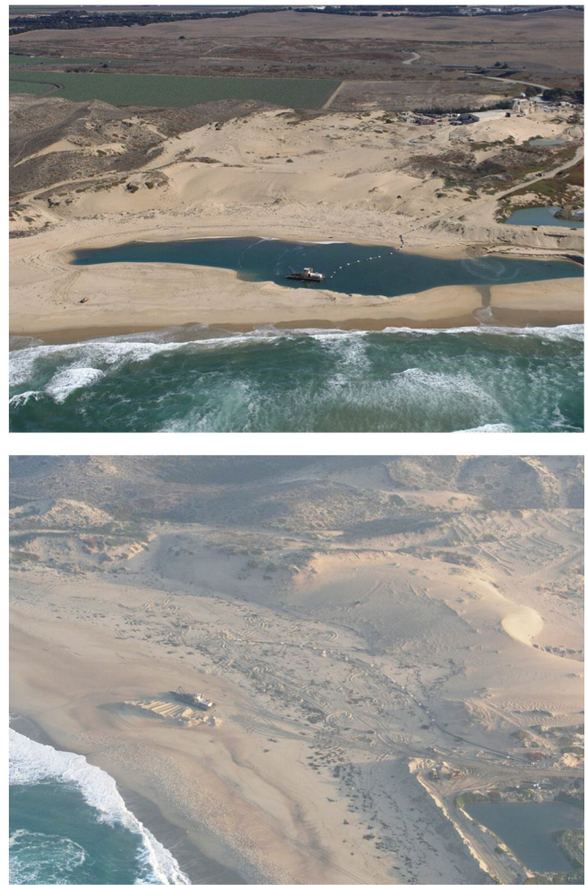
Fig. 12. Aerial photographs of dredge pond during operation in April 2005. Copyright 2005 Kenneth and Gabrielle Adelman, California Coastal Records Project, www.Californiacoastline.org (upper panel) and when dredge pond is filled with sediments in the winter (photo taken by Rob Wyland 15 January 2008) (lower panel).
