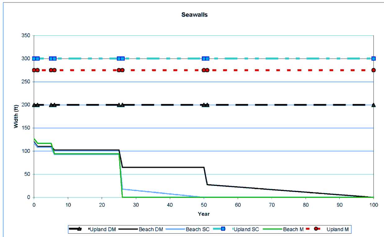
Figure 42 Effectiveness of seawalls at maintaining dry sand beach widths and upland property over time
