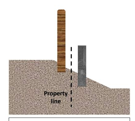
A fence or a wall is considered a separate fence or a separate wall when located on separate building sites
