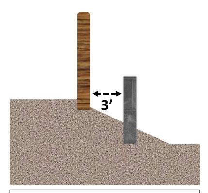
A fence or a wall is considered a separate fence or a separate wall when separated by a minimum of three feet
