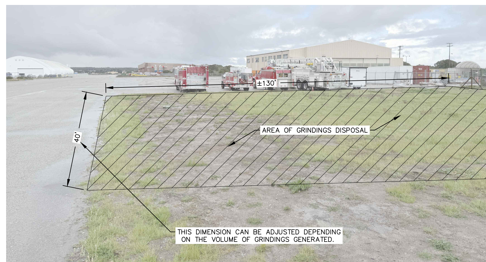
RECYCLED ASPHALT GRINDINGS PLACEMENT AREA
