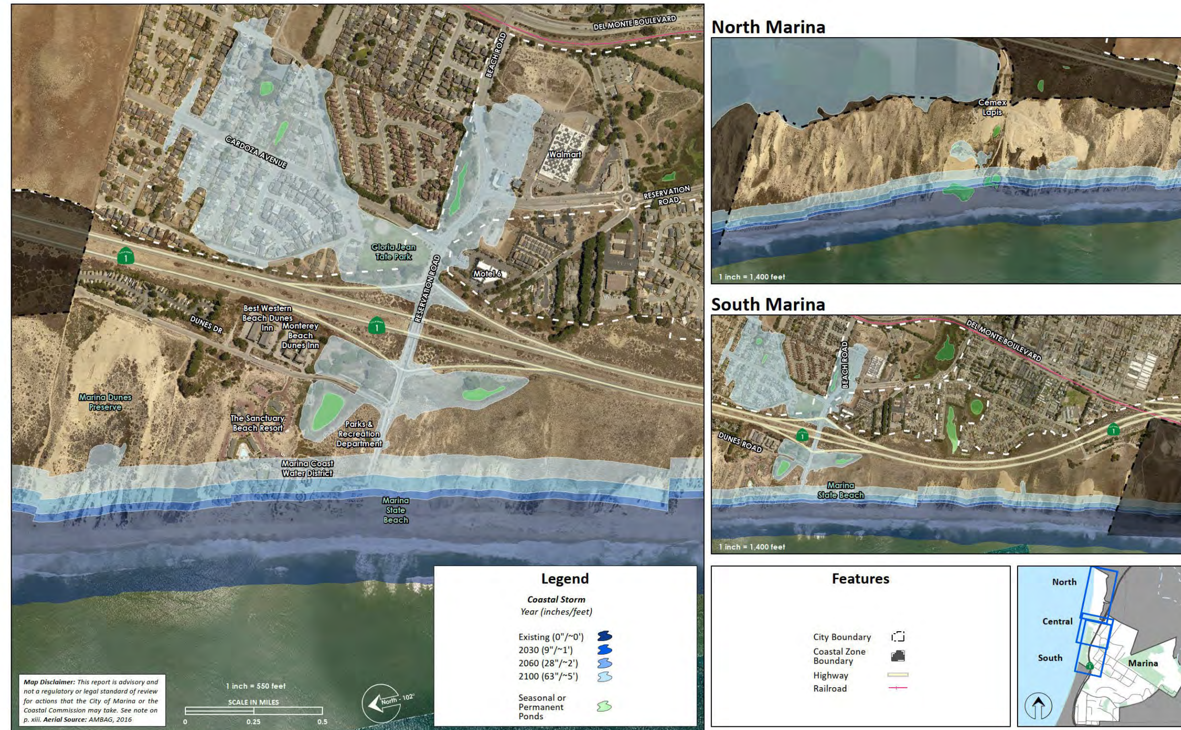
Figure 4-2. Projected Extent of Coastal Flood Hazards with 5 Feet of Sea Level Rise and a Major Storm Wave Event
